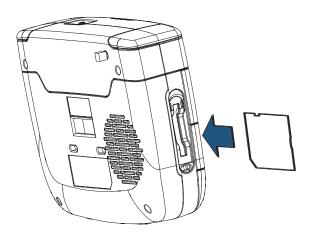
Peel back the rubber gasket to expose the memory card slot. Do not completely remove the rubber gasket.
